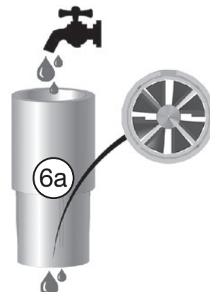
Fig. 5.18: Clean the measuring turbine under running water
