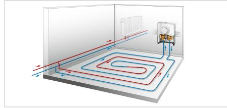
"Unibox TQ" Installation example including surface heating
