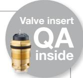
The thermostatic valves "AQ" limit the volume flow, for instance through a radiator, to a preset value. A complex calculation of the presetting values is no longer necessary. Only the required volume flows must be known. Control of the volume flow is carried out by the valve once the correct volume flow of the terminal unit has been set. This way, hydronic balancing of the system is carried out easily.
