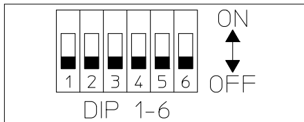
Illustr. 6: Setting of DIP switch
